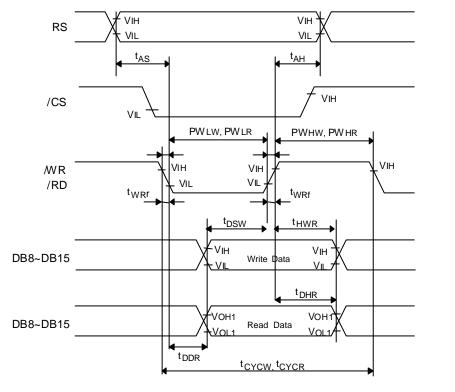
\*PWLw and PWLR are specified in the overlapped period when CS\* is low and WR\* or RD\* is low.
